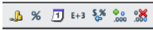
Figure 50: Number format icons. Left to right: currency, percentage, date, exponential, standard, add decimal place, delete decimal place.
